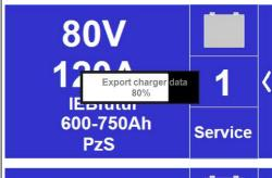
When the USB storage is plugged into the USB interface of the charger while the start display is active, the data is automatically exported to the main folder of the USB storage.
